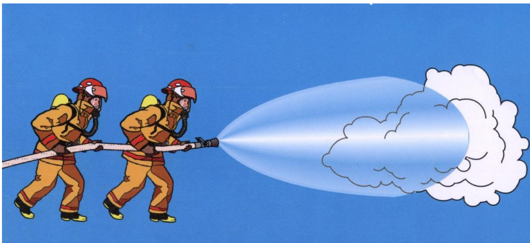
Fig. 2. Use of dispersion spray reduces the concentration of combustible gas
