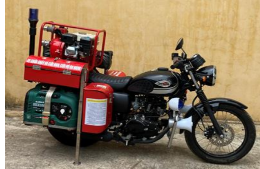
Fig. 2. Fire fighting and rescue motorbike
